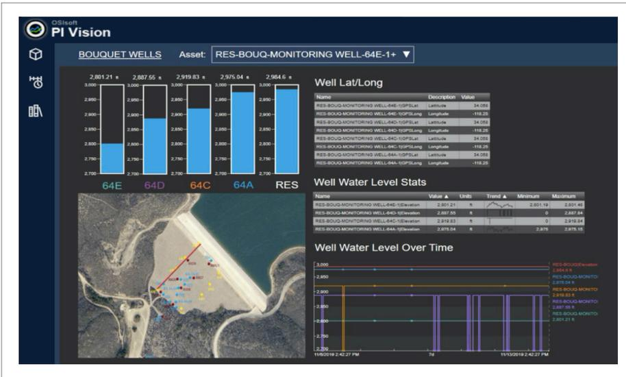
AVEVA PI Vision dashboard helps the LAPWD monitor the health of its dams at the Bouquet Reservoir in California by displaying important information about water levels in wells beneath the dams.
